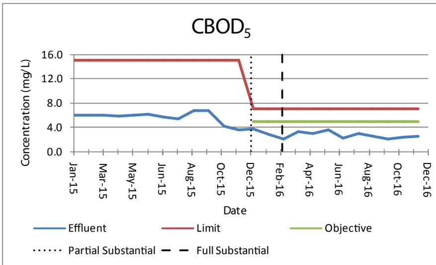
Figure 1. CBOD<sub>5</sub> effluent data.
