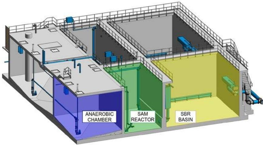
Schematic of the ISAM™ sequencing batch reactor.
