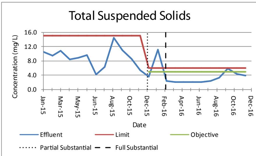
Figure 2. Total suspended solids effluent data.
